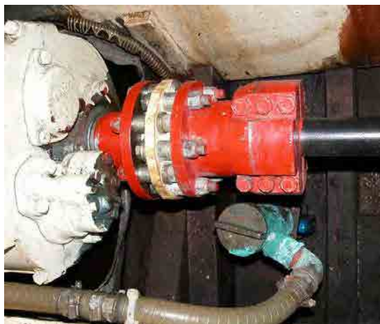
Coupling and Intake seacock with strainer
