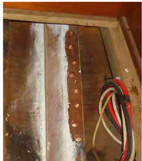
New ABracket backing timbers and bronze securing bolts fitted
