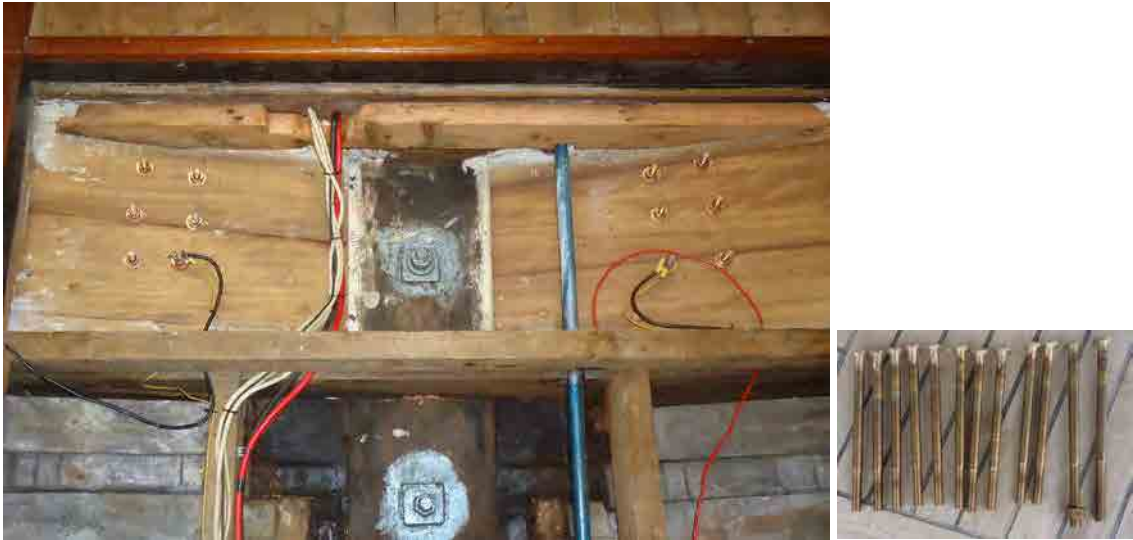
New ABracket backing timbers and bronze securing bolts fitted
